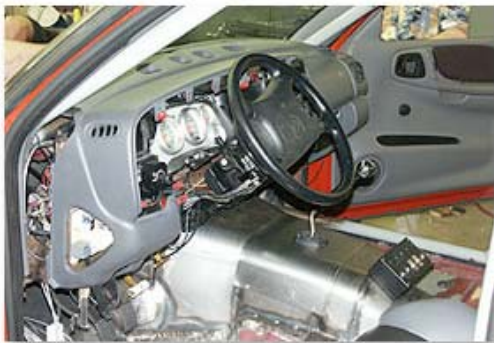
In-progress shot of interior. Large engine required relocating everything from the dash back further back into the cockpit. Dyno figures showed 393 hp @ 3800
